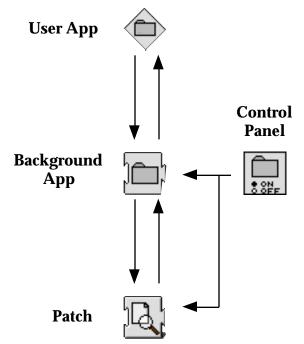
Figure 1. Components of our file system watcher.
